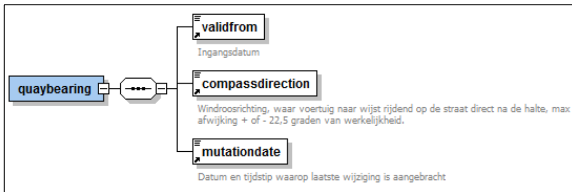
Figuur 13 XSD Quay-bearing
